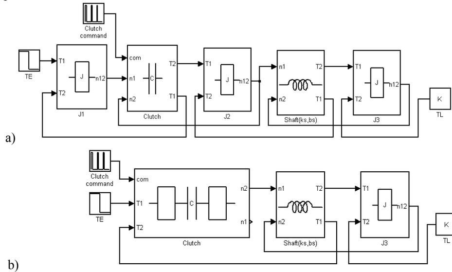
Fig. 7 Simulink top level diagram of a 3DOF powertrain model for: a) Coulomb, combined Coulomb-viscous friction and hyperbolic tangent clutch models; b) classic static model with switch and Karnopp model
