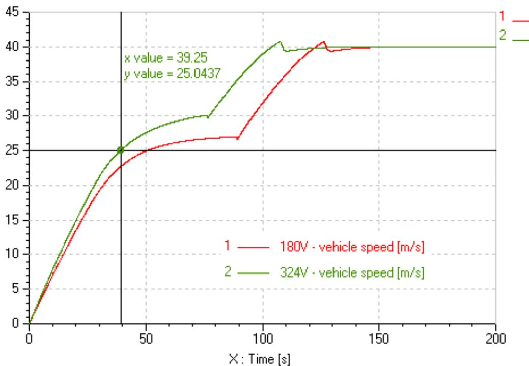
**Figure 10 – Acceleration (pure electric drive) for 180V and 324V battery**
