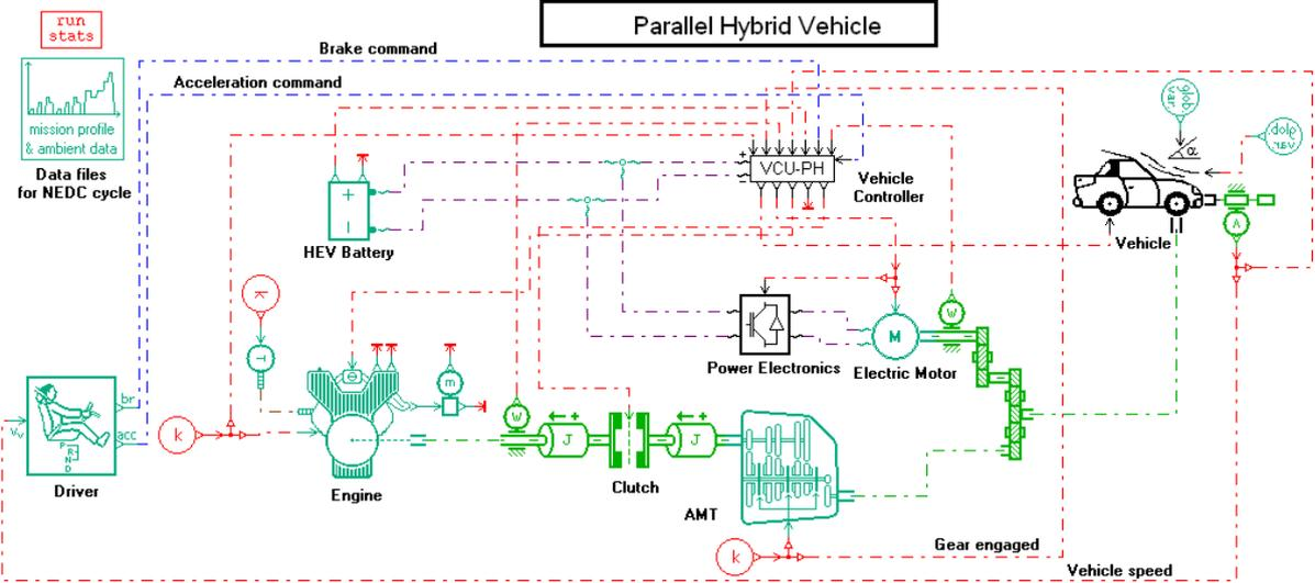
Figure 1 – Model sketch of hybrid car
