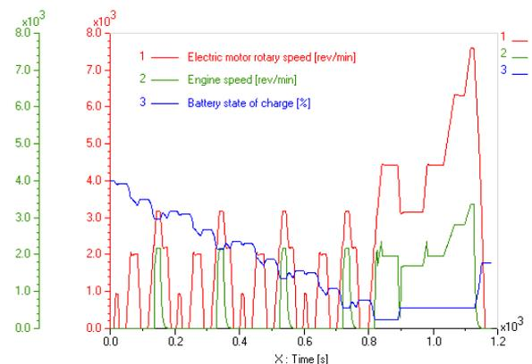
Figure 6 – Engine speed, electric motor speed and SOC[%]
