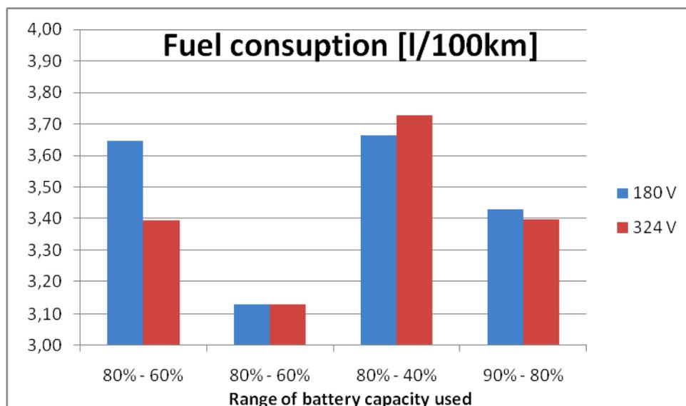
**Figure 7 – Fuel consumption values for the voltages analysed**
