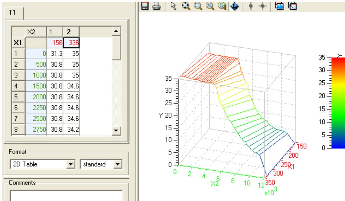
Figure 4 – Torque for electric motor [Nm] vs. revolution speed and voltage
