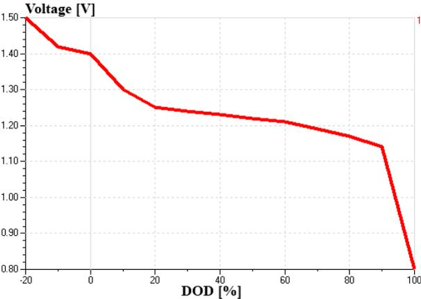
Figure 2 – Open circuit voltage for cell battery
