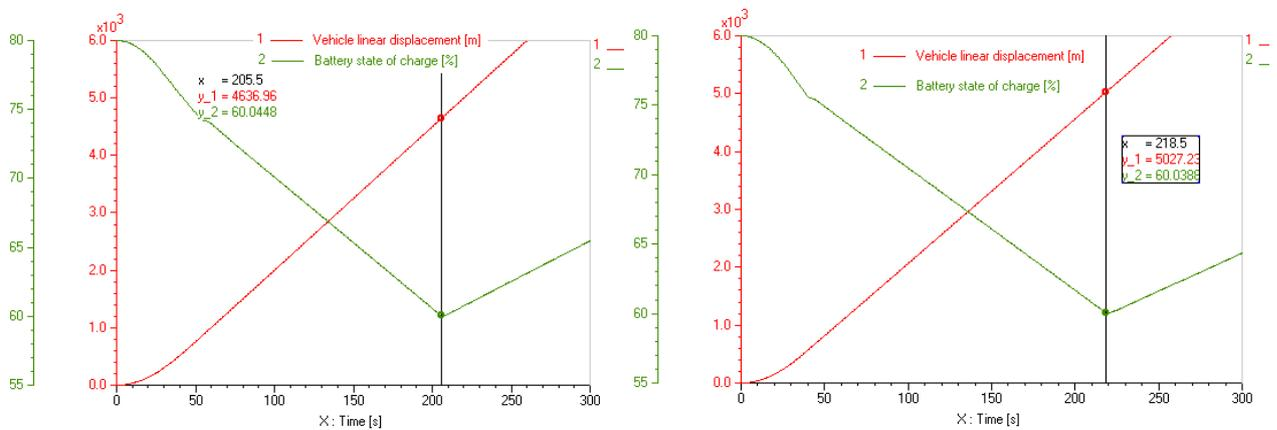
Figure 8 – Driving range at 90 km/h constant speed for 180 V, respectively 324V
