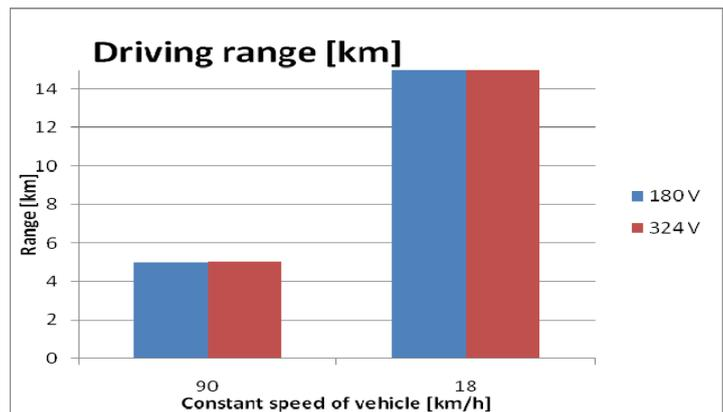
Figure 9 – Driving range for 90 and 18 km/h
