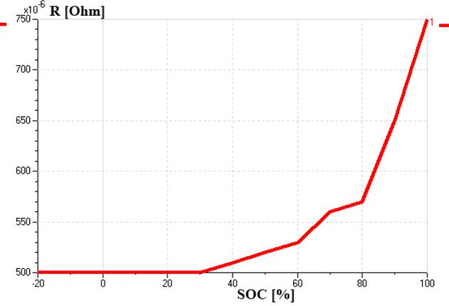
Figure 3 – Internal resistance for cell battery
