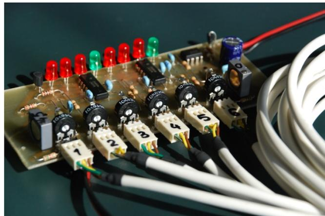
**Figure 3: Photo of simple battery management system**
