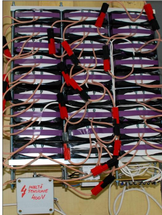
**Figure 1: 324V, 9.6Ah NiMH battery**
