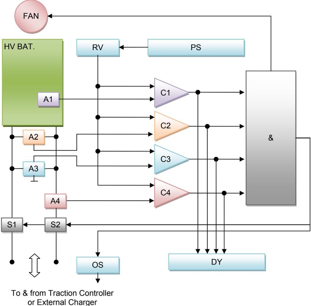
**Figure 2: Block diagram of a simple battery management system**
