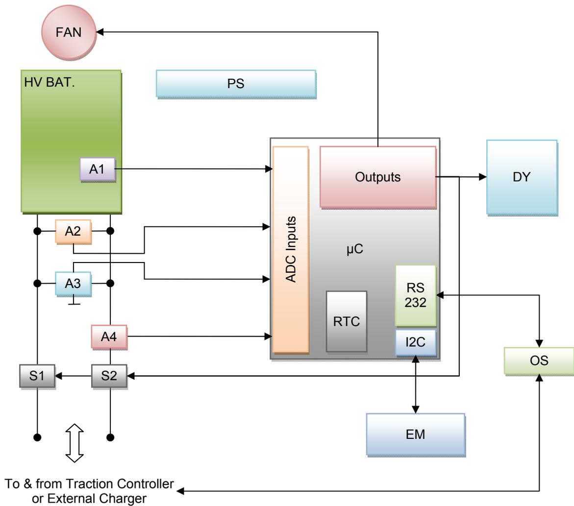
Figure 4: Block diagram of a simple battery management system
