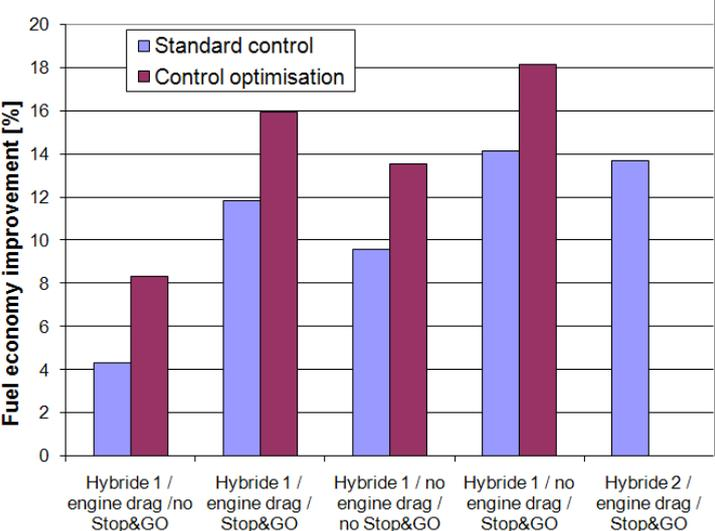
Figure 9: Comparative results of two different hybrid configurations
