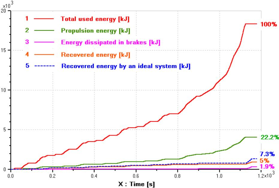
Figure 10: Energy analysis for the hybrid driveline
