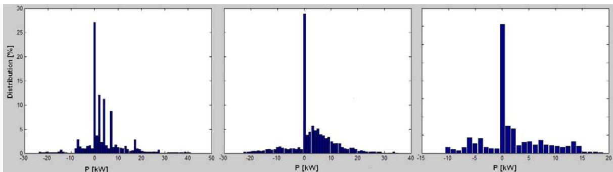
**Figure 5: Power distribution in NEDC, FTP-75, 10-15 mode driving cycles**
