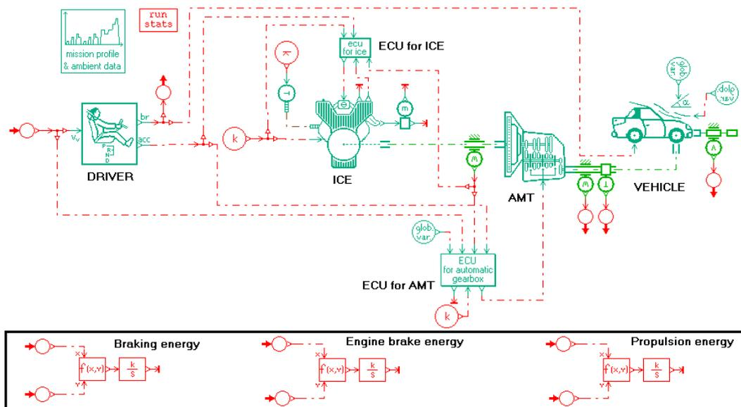
**Figure 1: Reference vehicle model**
