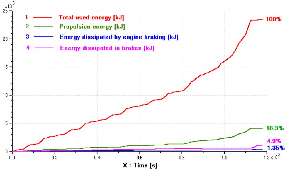
Figure 2: The energy balance of the reference vehicle model
