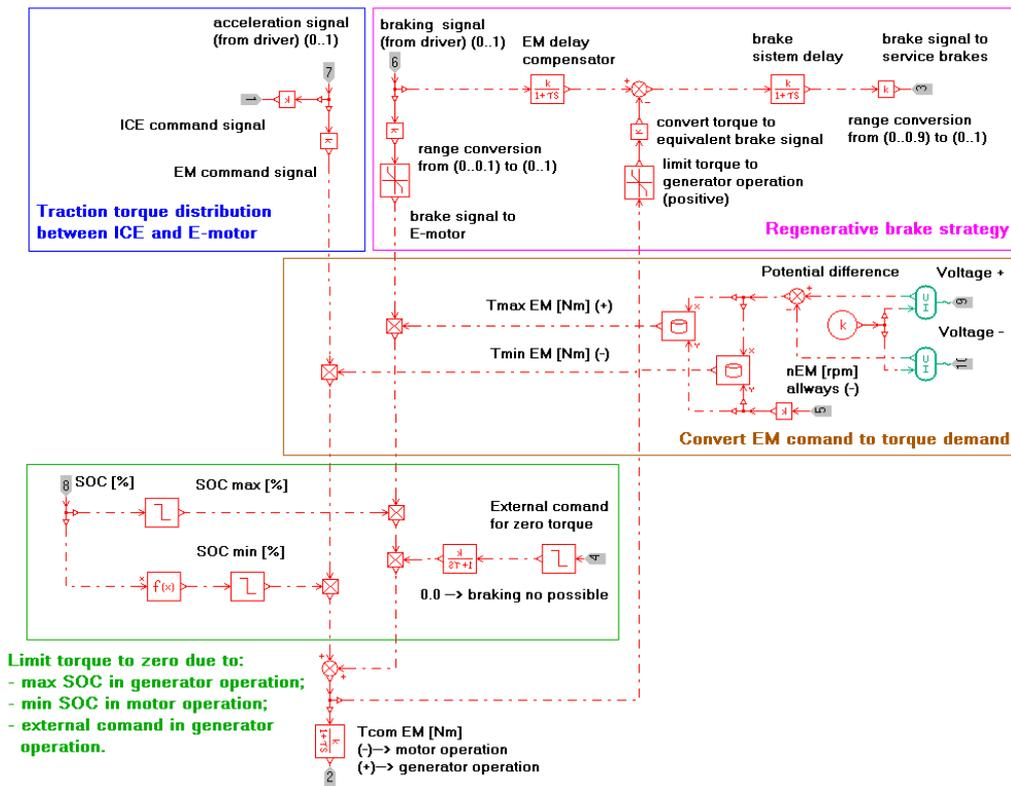
Figure 8: Hybrid command unit implemented using submodels from signal, control and observers library
