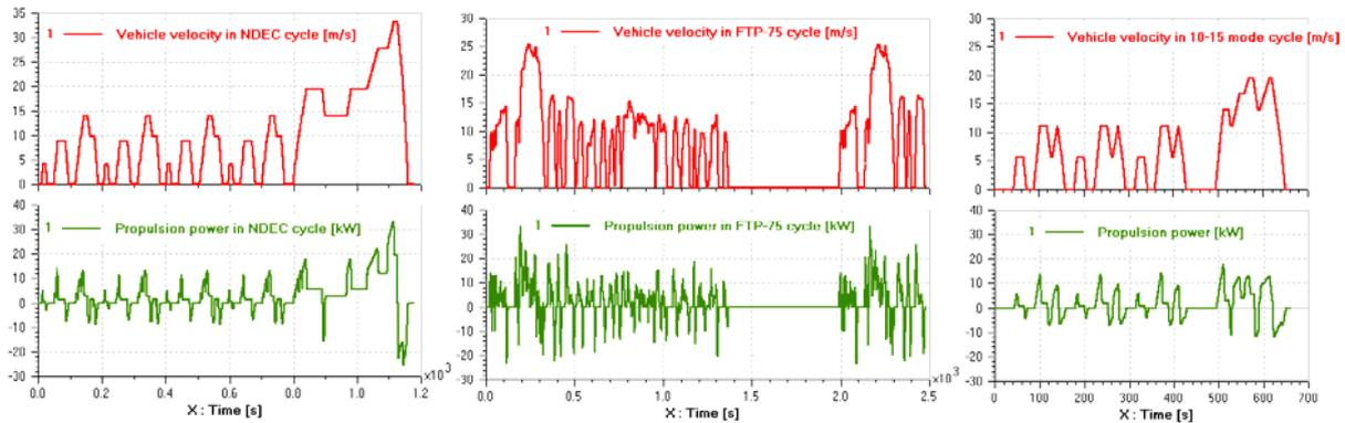
**Figure 4: Vehicle velocity and engine power evolution for the NDEC, FTP-75, 10-15 mode driving cycles**
