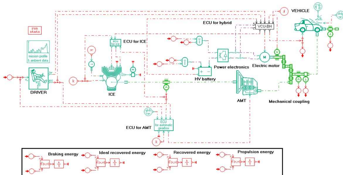
**Figure 7: Second hybrid configuration vehicle model**
