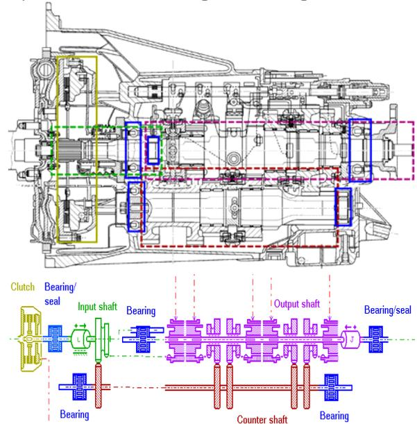
Figure 5: Detailed model of three-shaft gearbox
