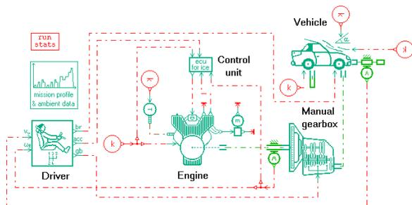
Figure 4: Powertrain model for fuel consumption
