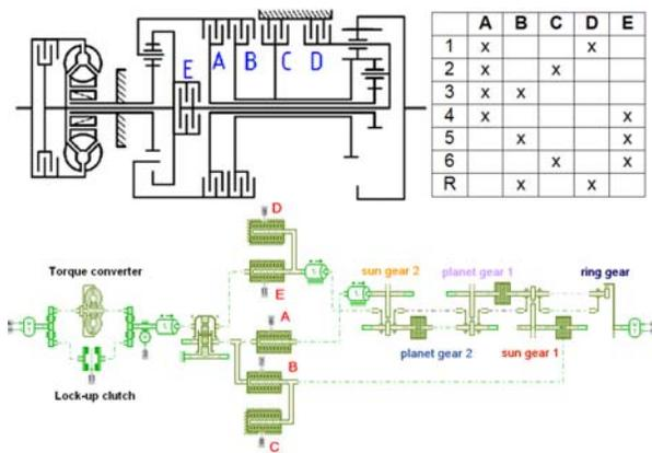
Figure 18: Advanced model of a 6 gear Lepelletier transmission with speed dependant losses
