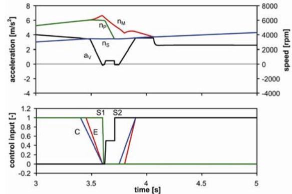
Figure 11: Simulation of a smooth gearshift process from 1st to 2nd gear at full throttle (AMT)
