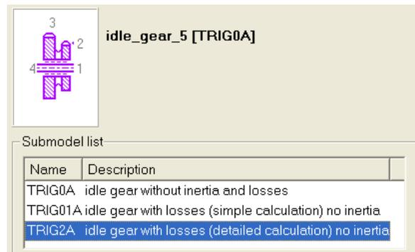
Figure 6: Submodels available for an idle gear
