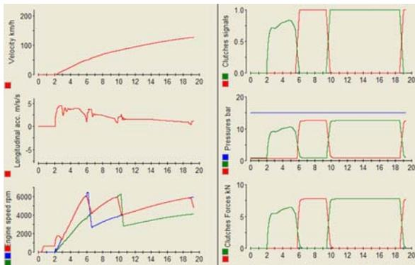
Figure 14: Simulation of WOT start of a DCT equipped vehicle on a RT platform
