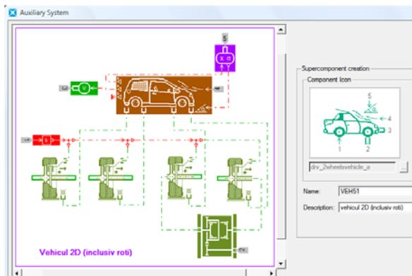
Figure 8: Supercomponent of a 2D vehicle with wheels and suspension
