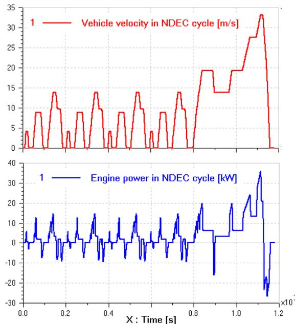
Figure 20: Vehicle velocity and engine power evolution for the NDEC driving cycle
