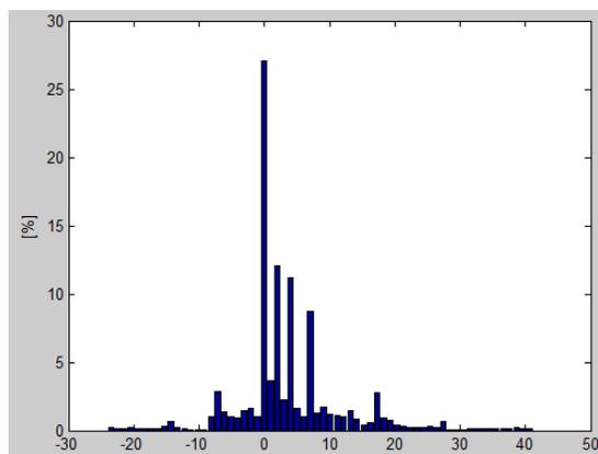
Figure 21: Power distribution in NEDC driving cycle
