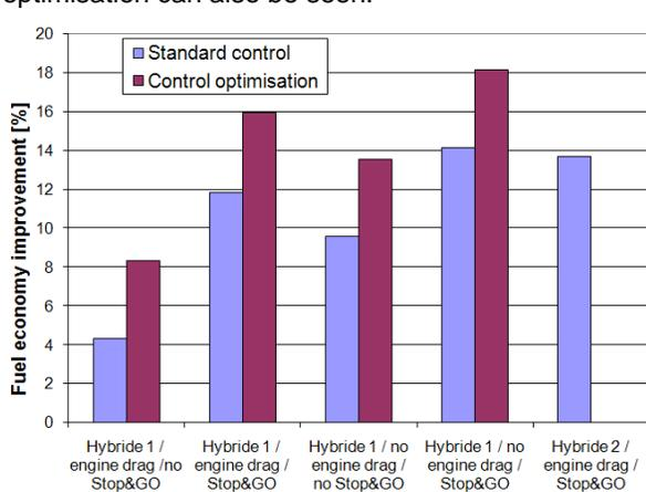
Figura 22: Comparative results of two different hybrid configuration
