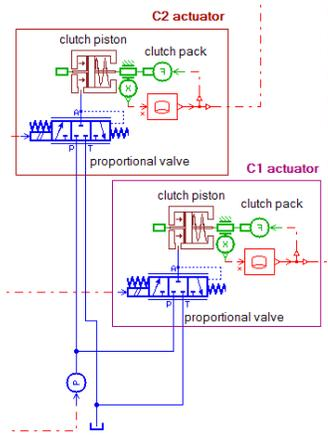
Figure 13: Simplified hydraulic circuit for DCT
