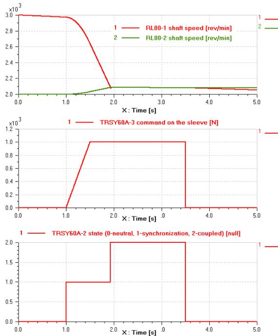
Figure 9: The synchronizations process in the new model
