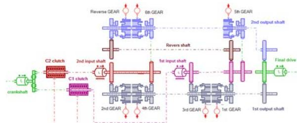
Figure 12: 6 gear DCT model
