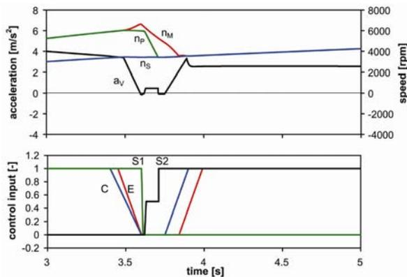
Figure 10: Simulation of a rapid gearshift process from 1st to 2nd gear at full throttle (AMT)
