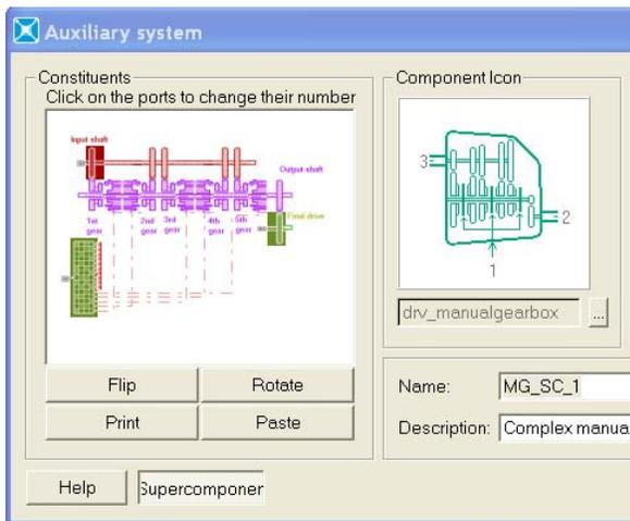
Figure 7: Supercomponent of a transaxle gearbox
