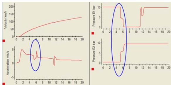
Figura 23: Improvement of acceleration profile by better control of coupling elements
