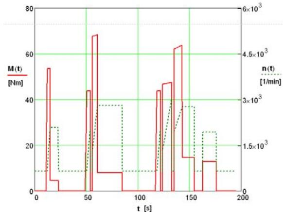
Figure 1: Variation of the transmission input torque and speed during a city driving cycle.
