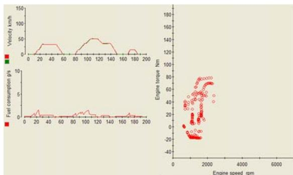
Figura 24: Fuel consumption and engine operating points for a imposed driving cycle
