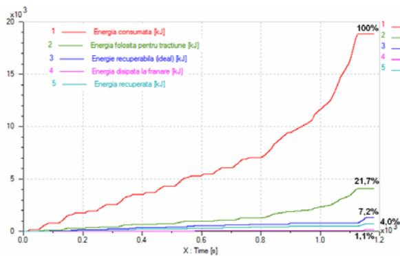
Figura 22: Energy analysis for the hybrid driveline
